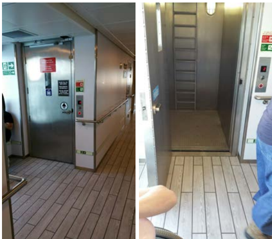
Elevators are only to be used when ferry is docked and not during crossings. Signs required informing passengers. Handrails needed for each wall of elevator
